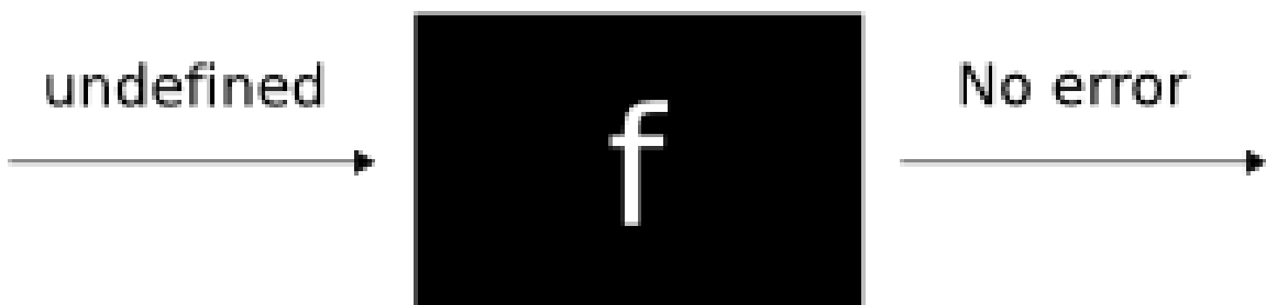
Figure 37: If f returns an error when passed undefined, it must be strict. Otherwise, it's lazy.
