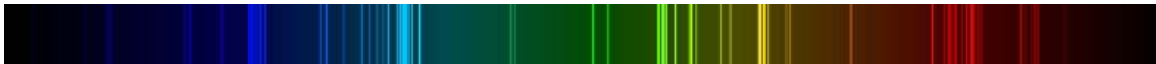
Figure 23: The emission spectrum of nitrogen gas. The spectral lines occur at specific wavelengths, showing the particle behavior of light.
