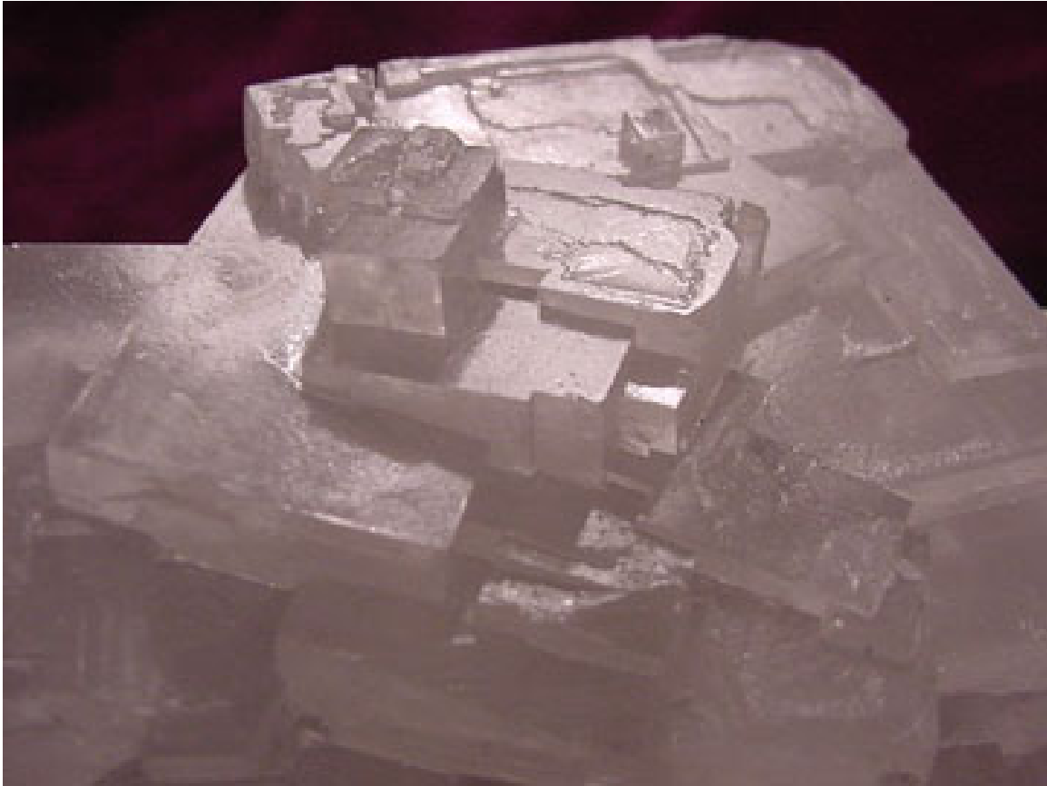
Figure 118: Halite, or rock salt, exhibits FCC packing.
