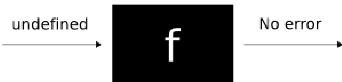
Abb. 37: If f returns an error when passed undefined, it must be strict. Otherwise, it's lazy.
