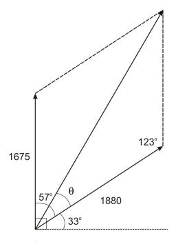
Since our two component vectors form a right angle, we can use trigonometric ratios to find their lengths (x and y).
