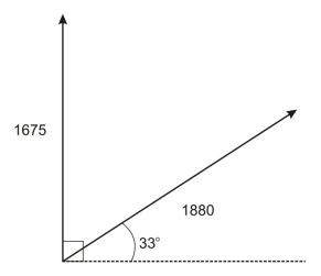
We are asked to find the resultant force and direction, which means we are dealing with vectors. In order to complete our diagram, we will need to connect our two vectors and draw in our resultant. We will refer to the magnitude of our resultant as x and the direction of our resultant as  $\theta$ .
