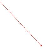
An object affected by this wind would travel in a southeast direction at 25 mph.
