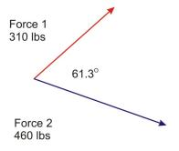
**Real-World Application:** Two forces of 310 lbs and 460 lbs are acting on an object. The angle between the two forces is 61.3°. What is the magnitude of the resultant? What angle does the resultant make with the smaller force?
