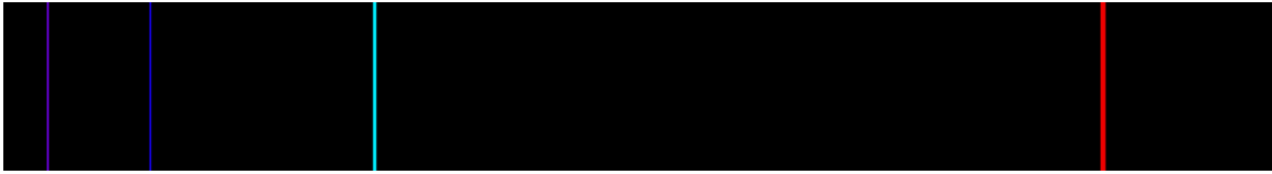
Figure 21: Visible emission spectrum of atomic hydrogen, containing four lines of the BALMER SERIES 16 .
