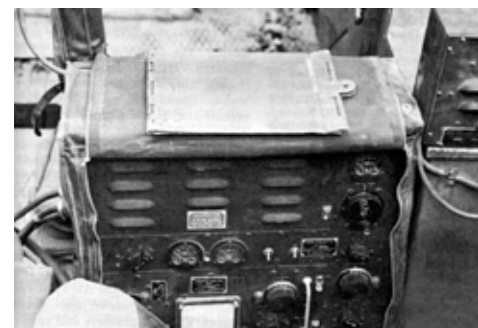
The jeep-mounted SCR-193 radio set provided Morse code and voice capability at a range of 25 to 100 miles, even while the vehicle was moving.
