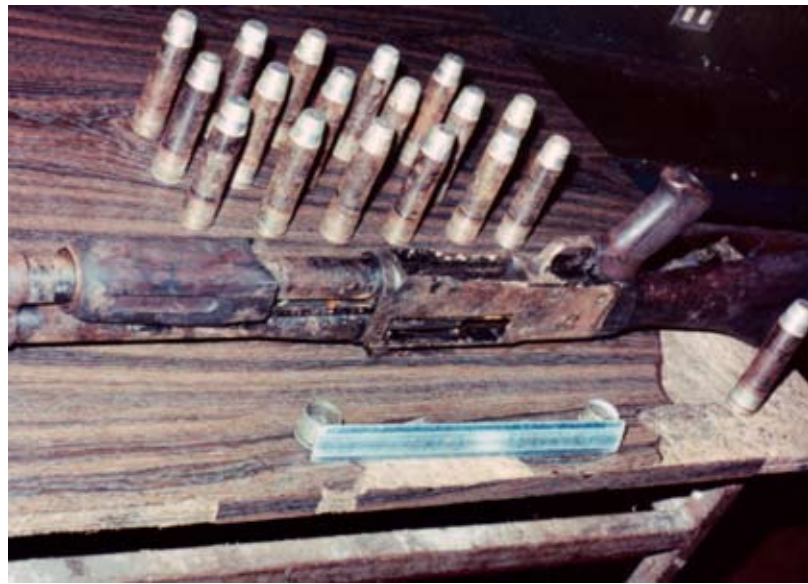
Homemade 12.7mm canon rifle fabricated from Soviet Mi-24 HIND-D attack helicopter chain machine gun breach block. It was abandoned by the Farabundo Marti National Liberation Movement after the September 1988 attack on El Paraiso.
