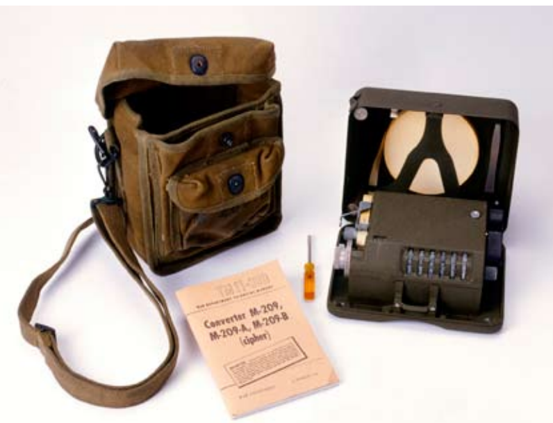
The M-209 cipher machine encoded and decoded messages in five-letter groups. Because the British were unfamiliar with the machine, the 112th sent cryptographic teams with the 6th Airborne Division to ensure continuity of communication.
