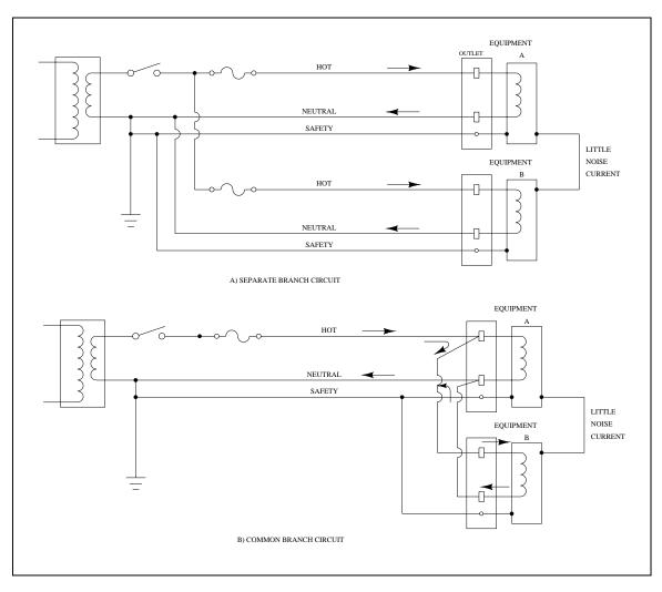
Figure 4-8. Properly wired ac distribution circuits for minimum ground noise
