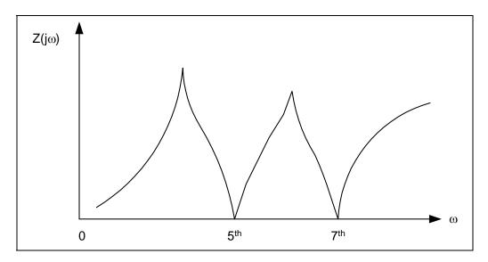
Figure 5-2. Impedance poles and zeros of tuned passive filter
