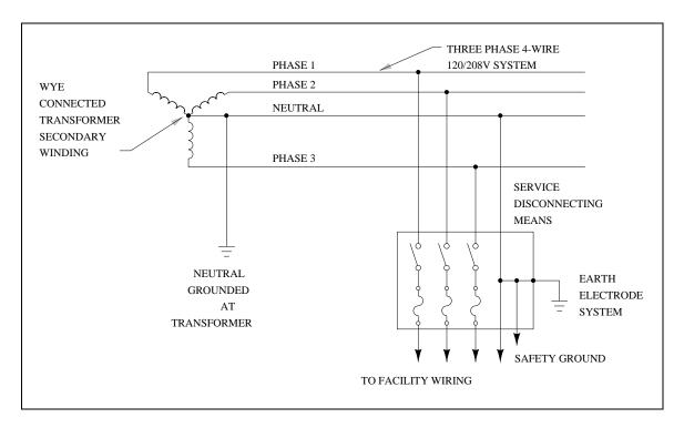
Figure 4-7. Three phase 120/208 Vac power system ground connections
