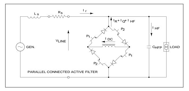
Figure 5-4. Active load current compensation
