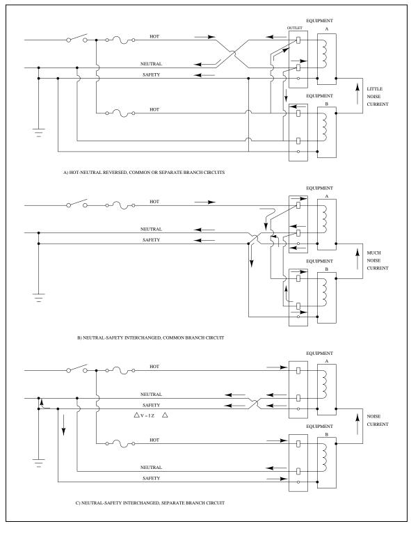
cables (including coax and other cable shields), and structural support members. Voltage drops associated with this return load current appear as common-mode noise sources between
