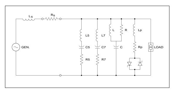
Figure 5-3. Tuned passive filter with static VAR control
