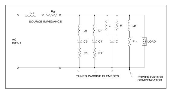
Figure 5-1. Tuned passive filter
