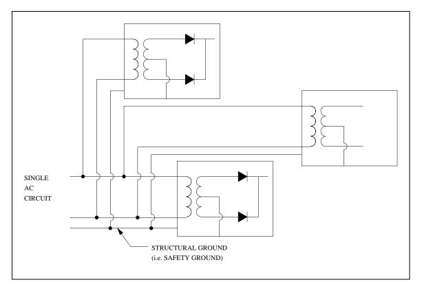
Figure 4-4. Basic grounding of a clustered system
