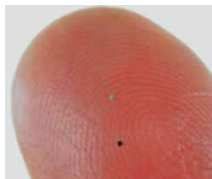
Hitachi \mu -chip (0.4 x 0.4mm)
