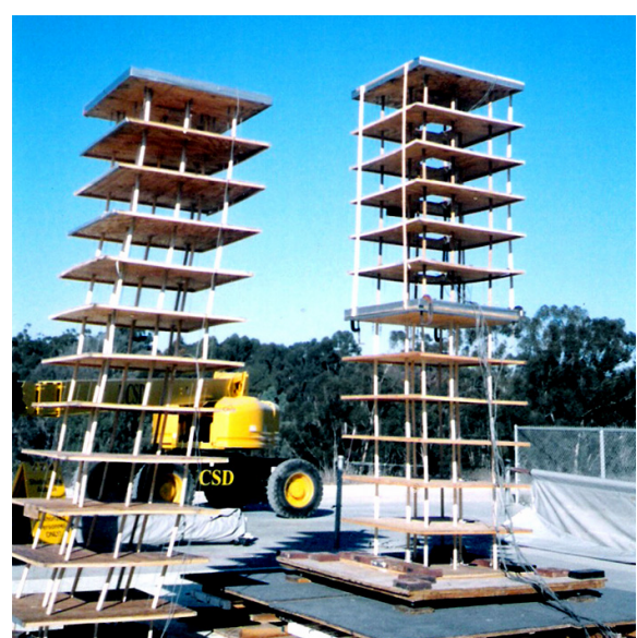
Concurrent shake table testing of two building models. The right model rests on base isolators, the left one is fixed to the platen [2] .
