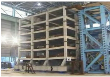
Snapshot from a shake-table destructive testing in Japan [1]
