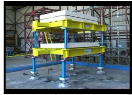
FPB [1] shake-table testing, Berkeley, CA.
