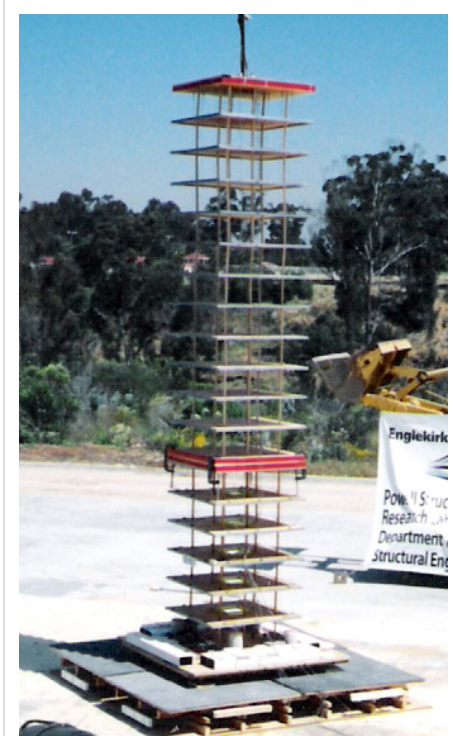
18-story model on earthquake protectors: shake-table test at UCSD outdoor facility.
