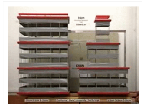
Shake-table testing of a regular building model (left) and a model with the vertical control (right) [1]
