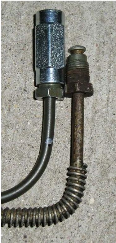
Partially assembled connector with ISO flare
