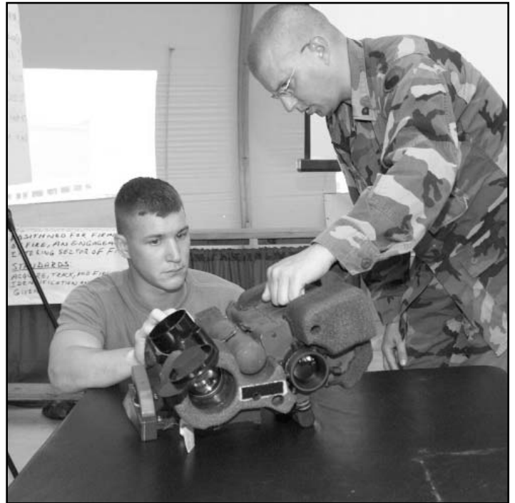
Photo by Sgt. Erin Viola Spc. Eric Gibbons (right) instructs Spc. Matthew Woyansky (left) on how to use a night tracking system that uses thermal imagery to detect the presence of the human form. The night tracking system is part of the tube launched optical wire guided weapon system, otherwise known as TOW.
