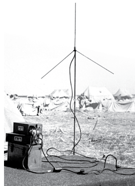
British S-phone air-ground radio.
