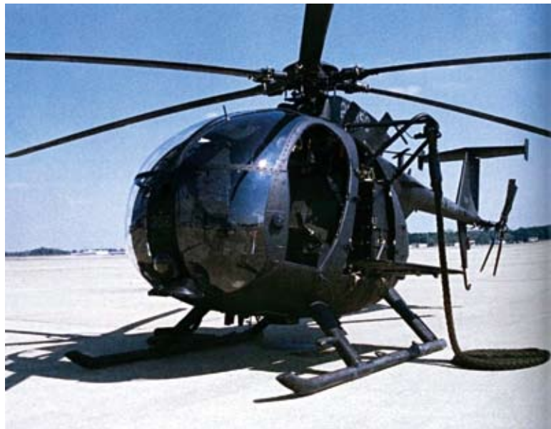
MH-6 "Little Bird" rigged for a fast-rope insertion.
