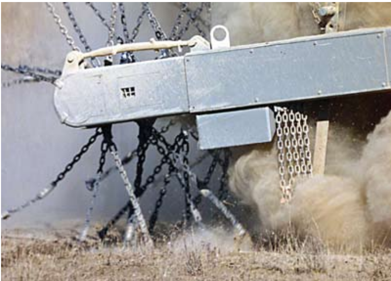
An effective mine-clearing device, the Aardvark was used extensively to prepare the area for occupation.
