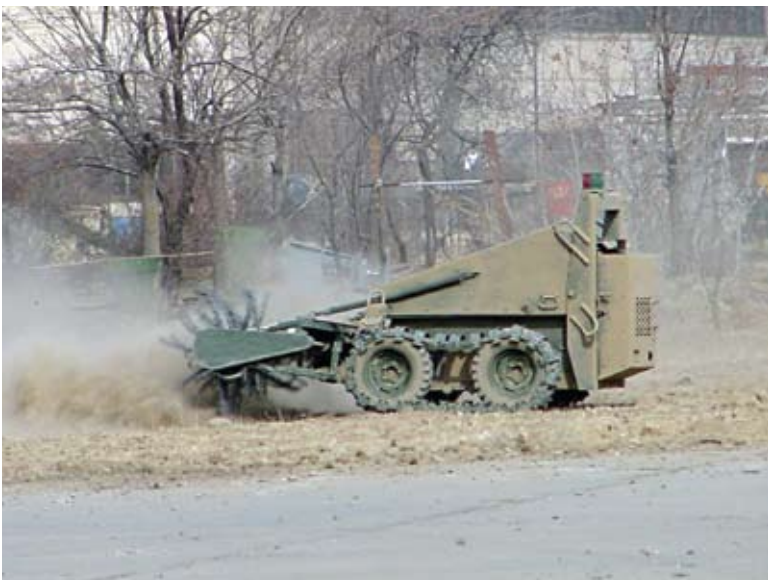
A smaller, remote-controlled mine-clearing vehicle, the Mini-flail, was operated by the Jordanians at Bagram.
