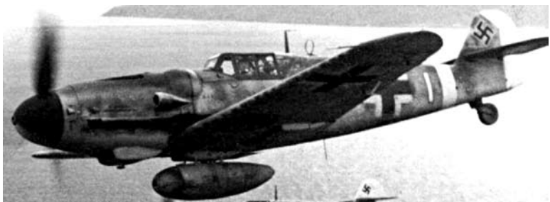
German Messerschmitt ME-109G fighter plane with belly tank to extend its operating range.
