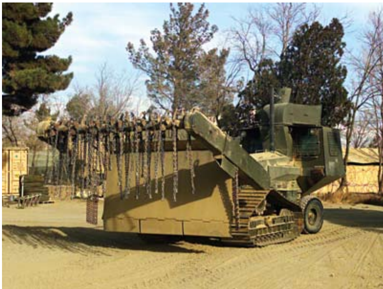
The Aardvark mine-clearing vehicle used a chain-flail system to detonate the mines. It was operated in Bagram by the Norwegian contingent.
