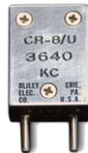
Actual size of a frequency crystal for a Type A Mark III radio.
