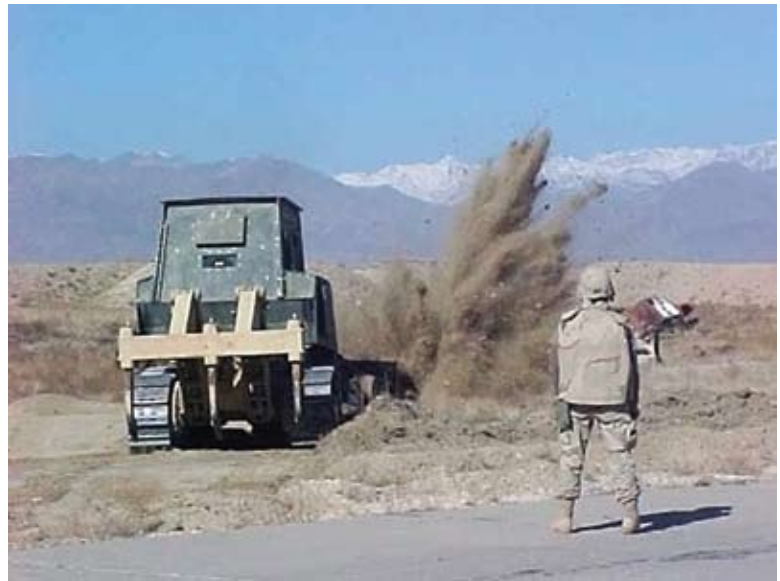
The D9 Mobile Combat Armored Bulldozer was the primary mine-clearing vehicle in use by the 92nd Engineer Battalion.
