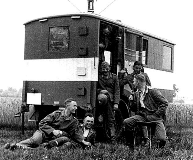
The Germans normally employed these radio direction-finding trailer vans in threes to triangulate radio transmission sites. Linked to these radio-tracking units were stand-by teams of Gestapo and SD (Sicherheitsdienst, or Security Service) agents and soldiers to trap unsuspecting RTOs.
