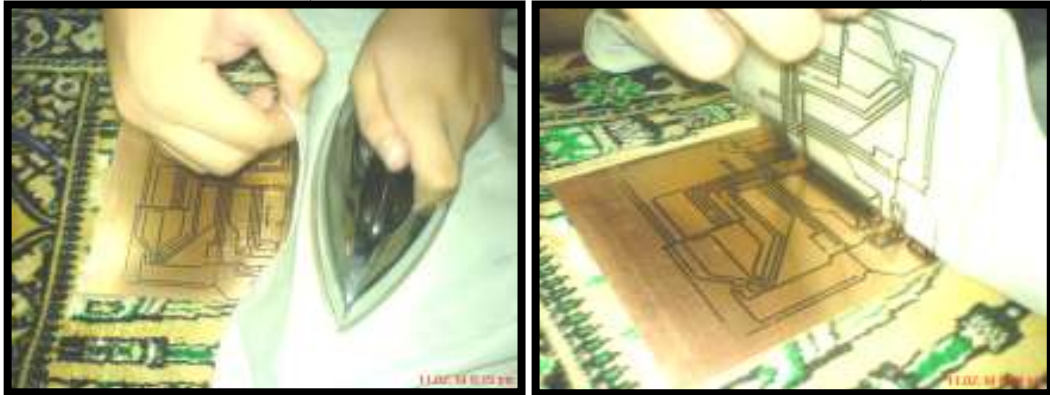
Figure 3.20: Ironing the Layout Method
