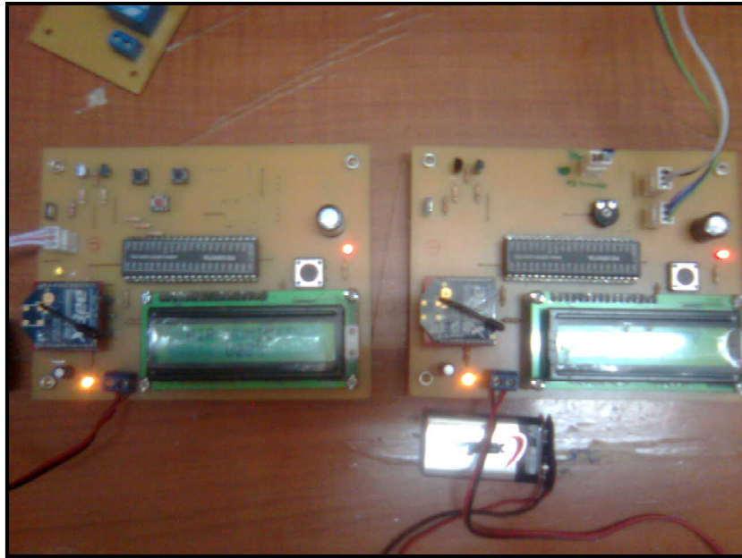
Transmitter and receiver board
