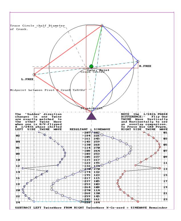
Below is Twine at -90 units of Pivot to Crank (EB\_Elastic)
