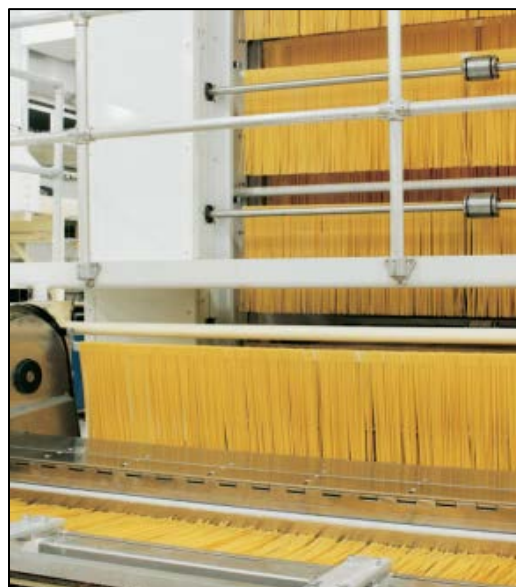
Stripper taking pasta off drying stick and getting ready for trimming to length. Multi-level accumulator in background. Photograph courtesy of DEMACO.
