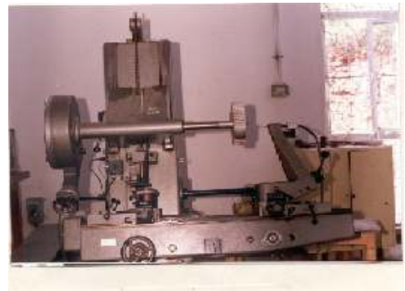
Fig: 4 Propeller Manufacture by Point Drilling
