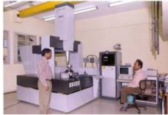
Fig:2 Inspection of Propeller on CMM
