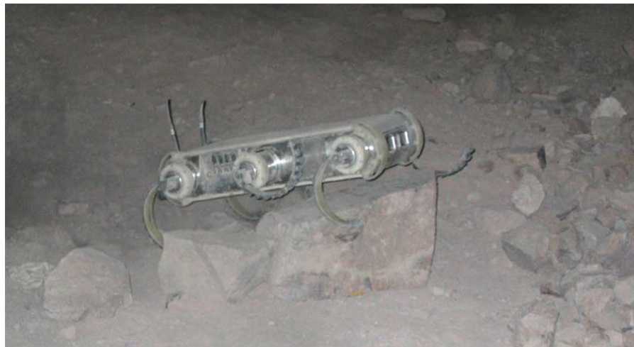
Figure 23: Bio-inspired hexapod, RHex, emulates cockroach-like locomotion to traverse difficult terrain.
