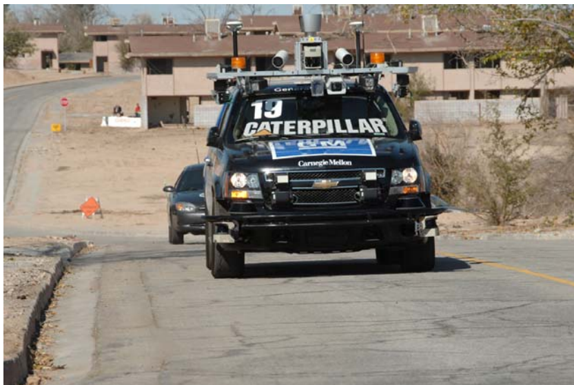
Figure 22: Tartan Racing's (Carnegie Mellon University) "Boss," the first place finisher in the DARPA Urban Challenge, on the course.
