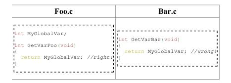
In the example above, the variable MyGlobalVar is visible inside the file Foo.c, but is not visible inside the file Bar.c. To make MyGlobalVar visible inside all project files, we need to use the extern keyword, which we will discuss below.
