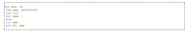
When you see a comparison, followed by a je or a jne, **reverse the condition of the jump to recreate the high-level code.** For jump-if-greater (jg), jump-if-greater-or-equal (jge), jump-if-less-than (jl), or similar instructions, it is a bit different than simply reversing the condition of the jump. For example, this assembler code:
