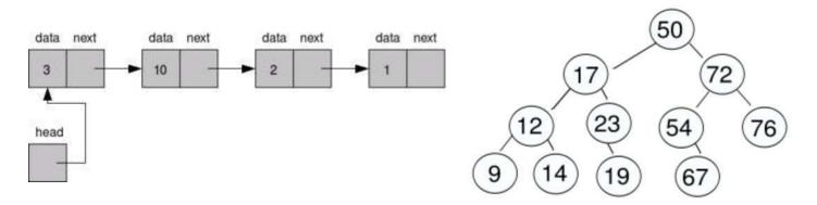
Each node in a linked list or a binary tree contains some amount of data, and a pointer (or pointers) to other nodes. Consider the following asm code example:
