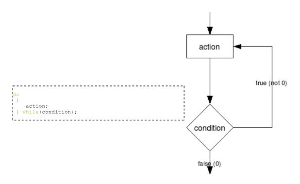
What does this loop do? The loop body simply executes, the condition is tested at the end of the loop, and the loop jumps back to the beginning of the loop if the condition is satisfied. Unlike **if** statements, Do-While conditions are not reversed.
