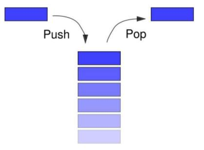
**esp** register. The stack "grows" downward, from high to low memory addresses, so values recently pushed onto the stack are located in memory addresses *above* the esp pointer. No register specifically points to the bottom of the stack, although most operating systems monitor the stack bounds to detect both "underflow" (popping an empty stack) and "overflow" (pushing too much information on the stack) conditions.
