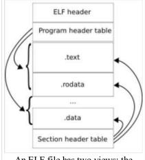
An ELF file has two views: the program header shows the *segments* used at run-time, while the section header lists the set of *sections* of the binary.
