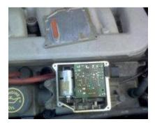
2. Second, there is supposed to be a white plastic screw holding on the transistor (notated on MY board by the "2" with the triangle. Your's might not have this). Remove this white plastic screw, discard. Then remove the five screws holding on the board to the housing. Now, pull slightly upwards with the black connector. The board and motor should come free.
