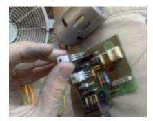
4. Remove the old transistor and put the new one in. Make sure it sits the exact same way, with the hole lined up to the one in the board.
