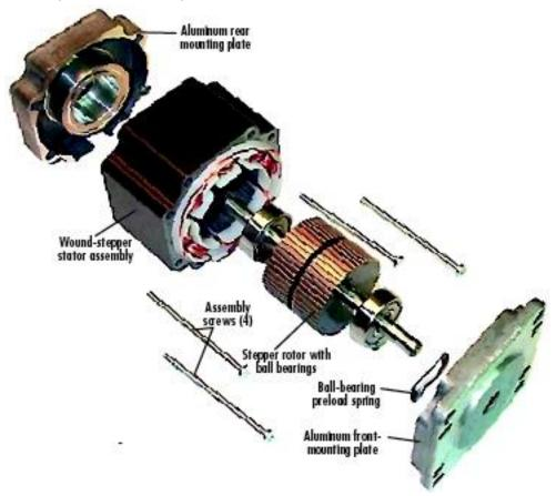
This is what actually gives the motor its 'steps'. By charging and releasing magnets on the stator in sequence you can get the position of the rotor to line up on the individual steps around a single revolution of the motors movement. Each ridge on the stepper rotor is an individual step and the number of steps a motor is capable of is the number of ridges around the circumference of the rotor.
