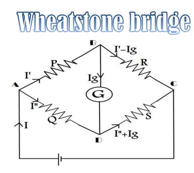
Wheastone bridge is an instrument used to messure unknown resistance amounn 3 resistances. It consis of 4 resistances P,Q,R & S.
