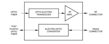
The RC200A converter contains, within it, two opto-electric conversion sub-systems.
