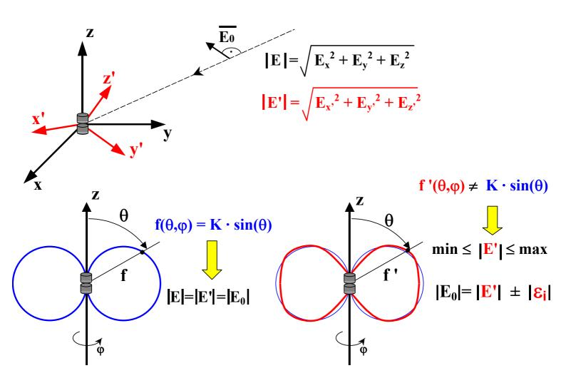
If omnidirectional antennas are not used, deviation from this characteristic causes a measurement error that cannot be corrected, since normally neither the propagation direction nor the polarisation of the field to be measured are known.
