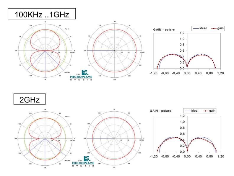
As the frequency increases, and in particular above 2.5 GHz (out of band), the characteristic radiation diagram distorts. It is therefore not possible to make correct measurements out of band due to the antenna's loss of omnidirectional capability.
