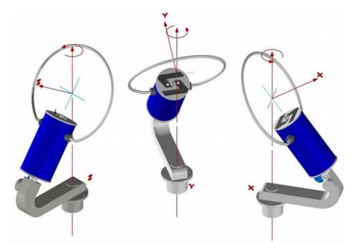
There is of course no need for one of the three measuring directions to be vertical, since the sensor is capable of operating with any spatial arrangement of its axes. In particular, this enables the sensor to be set up along three mutually orthogonal directions, by simple rotation through 120° round a special axis (ortho-angle).
