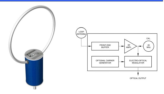
Sensor FP030H consists of an active loop antenna, powered by internal rechargeable batteries, sensitive to the magnetic field component orthogonal to the plane containing the detecting loop.
