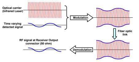
The electrical signal thus obtained can be picked up by means of a common RF cable and sent to a spectrum analyser.
