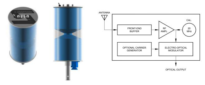
The FP2000 sensor is an active, omnidirectional dipole receiving antenna, powered by internal rechargeable batteries, sensitive to the electric field component parallel to its axis of symmetry.
