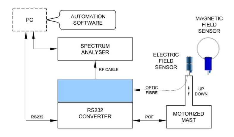
The measurement system consisting of a sensor, converter and spectrum analyser allows maximum operating flexibility when connected to a personal computer (PC) and used in conjunction with a motorised tripod specifically designed for the antenna.
