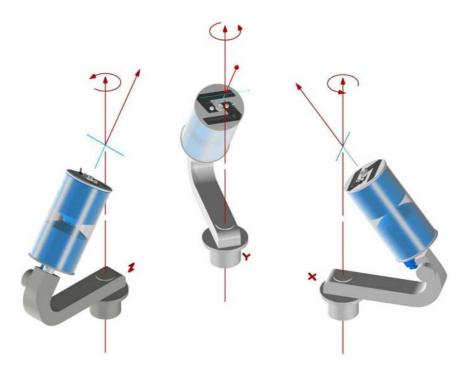
There is of course no need for one of the three measuring directions to be vertical, since the sensor is capable of operating with any spatial arrangement of its axes. In particular, this enables the sensor to be set up along three mutually orthogonal directions, by simple rotation through 120° round a special axis (ortho-angle).
