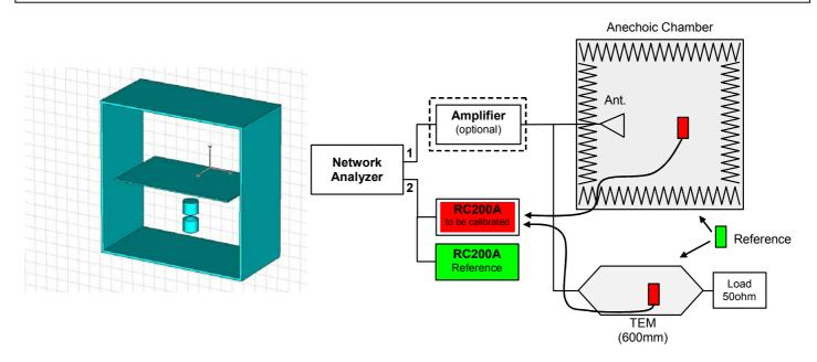
The procedure for calibrating the sensor and its accessories (converter and optical fibre) is based on the method of replacing the device being calibrated with a sample of identical model with known characteristics, calibrated in an EA accredited laboratory.
