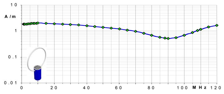
The signal sent to the spectrum analyser must emerge from the background noise appearing on the analyser screen. The level of the background noise therefore determines the minimum amplitude of signals that can be safely detected by the system. The chart below shows the **noise level** as it appears on the screen of a spectrum analyser connected to an FP030H, with different RBW settings. Note that the noise power is roughly proportional to the Resolution Band Width used.
