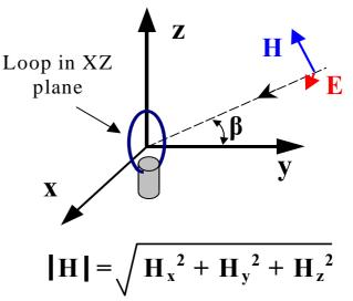
the converter is proportional to  $|\mathbf{H}| \cdot \sin \beta$ . To reconstruct total amplitude of the incident magnetic field it is therefore simply necessary to take three measurements, adjusting the sensor so that the loop plane is set up along three mutually orthogonal directions.
