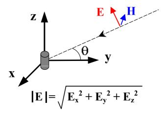
To reconstruct total amplitude of the local electric field, it is therefore simply necessary to take three measurements with the axis of the sensor set up along three directions mutually orthogonal to each other.
