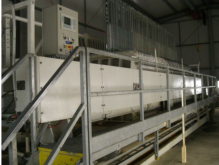
Figure 25.13: Sand processing Mill, near Provodin, Czech Republic. Water is used to wash mined sand, then is drained into tanks, filtered, and recycled. (17)
