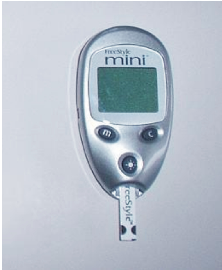
Figure 21.12: This is one type of meter used by people with diabetes to measure their blood sugar. Modern meters like this one need only a drop of blood and take less than a minute to use. (25)
