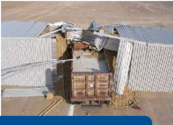
Determining impact resistance. A dump truck crashed into a Metalith barrier during testing.
