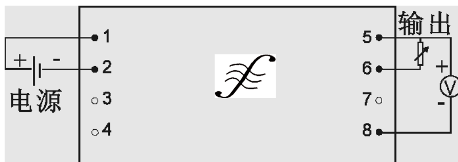
GRBXXXX- B B Model Connection Diagram (bottom view)
