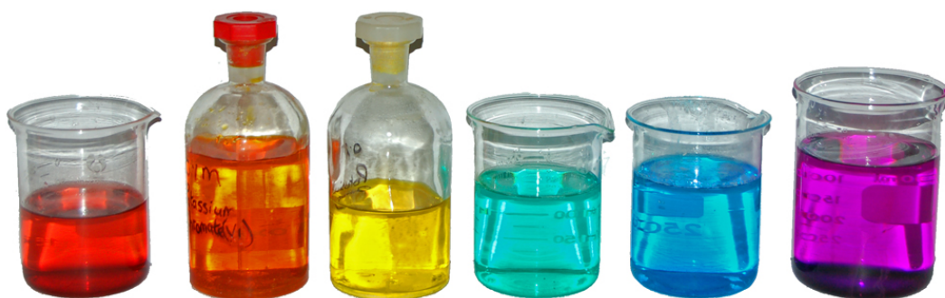
Figure 168: Left to right: cobalt(II) nitrate (red); potassium dichromate (orange); potassium chromate (yellow); nickel(II) chloride (green); copper(II) sulfate (blue); potassium permanganate (purple).
