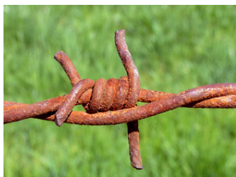
Figure 132: This iron wire has taken years to become rusty.
