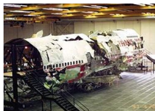
The wreckage of TWA 800, reconstructed for the investigation
