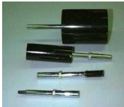
A range of ionisation chambers of different volumes used for measuring radiation exposure.
