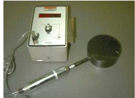
An exposure meter used in radiography.
