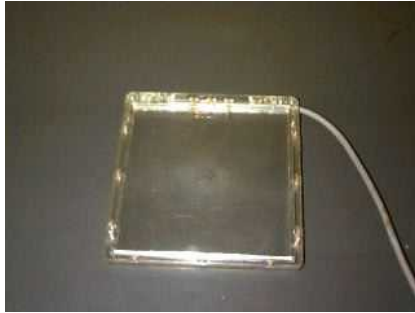
An exposure-area product detector used in radiography.
