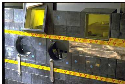
Another view of the Pb shielding surrounding a laminar flow cabinet.
