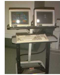
The image acquisition and processing console of a dual-headed gamma camera.
