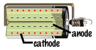
to flow from the anode (the negative part of the battery) through the external bulb connection and back to the cathode (the positive part of the battery).
