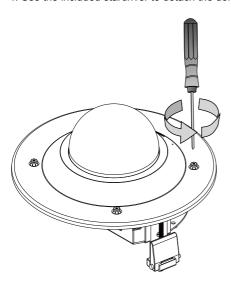
5. Install camera to the recessed-mount bracket by driving 2 screws.
