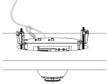
You may also use a cable tie to secure cables to the anchor point on top.
