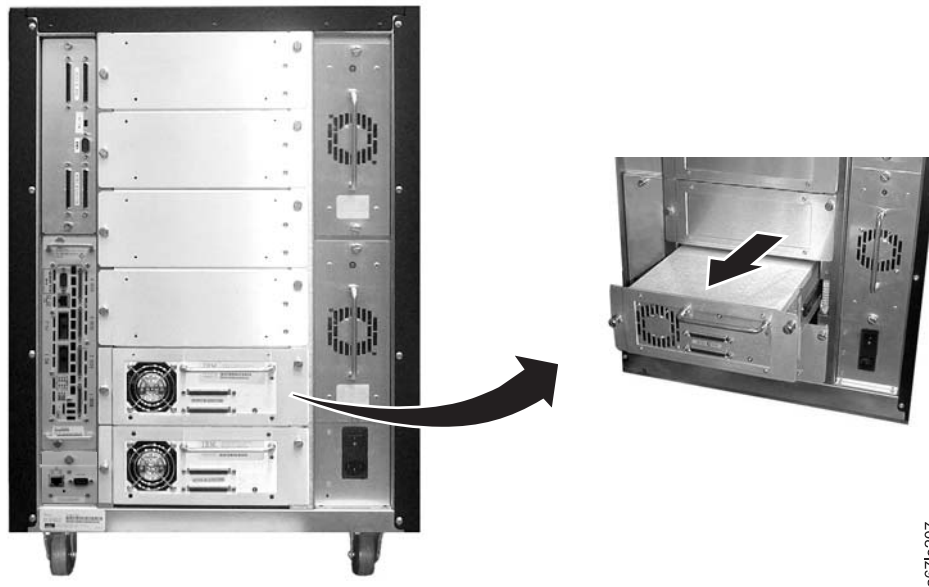
Figure 1-4. SCSI Ultrium 1 Tape Drive in the Ultrium Scalable Tape Library. The tape drive is contained in a removable drive sled. The view is from the rear of the library.
