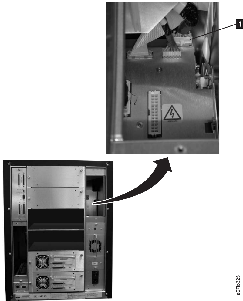
Figure 8-36. Disconnecting the accessory bay cable from the power distribution PCBA. Figure shows a converted library.
