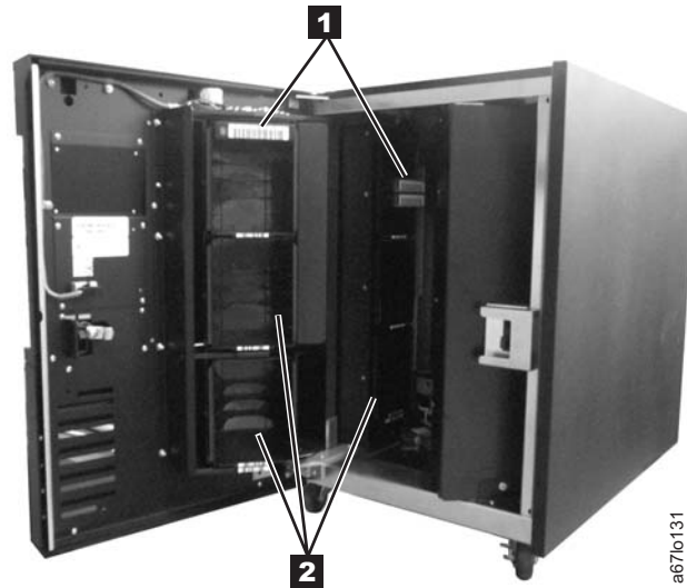
Figure 14-16. Removing cartridges and magazines
