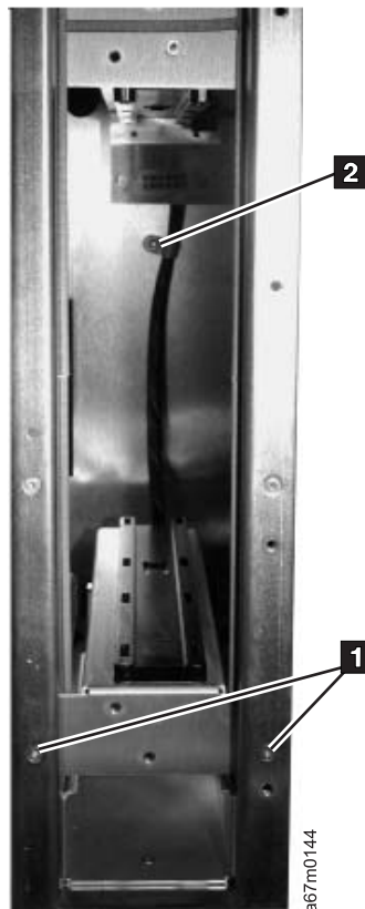
Figure 8-28. Removing the Lower Fibre Channel Bracket Sub-Assembly
