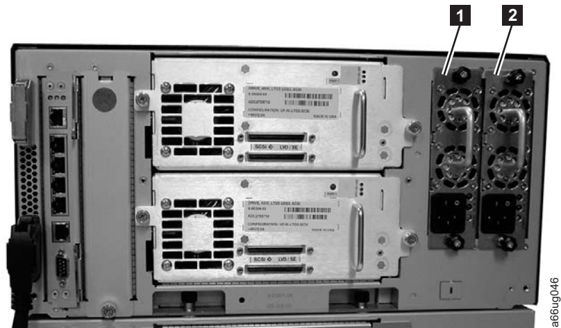
Figure 1-8. Power supply location coordinates
