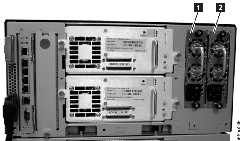
Figure 11-1. Power supplies in a control module
