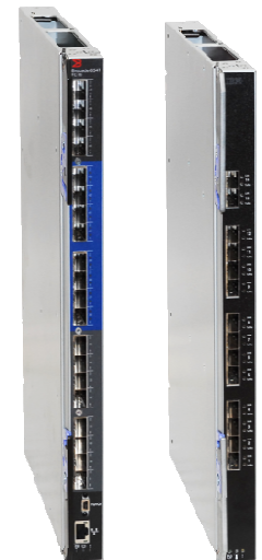
IBM Fiber and Ethernet Switches
