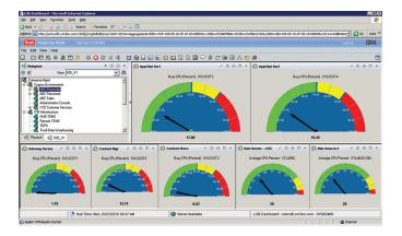
Tivoli software provides a simple, configurable dashboard view of the utilization across the various Cognos 8 BI infrastructure components to highlight degrading performance that needs attention.
