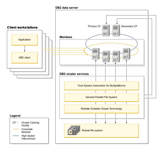
Db2 cluster services provide essential infrastructure for the shared data instance to be highly available and to provide automatic failover and restart as soon as the instance has been created.
