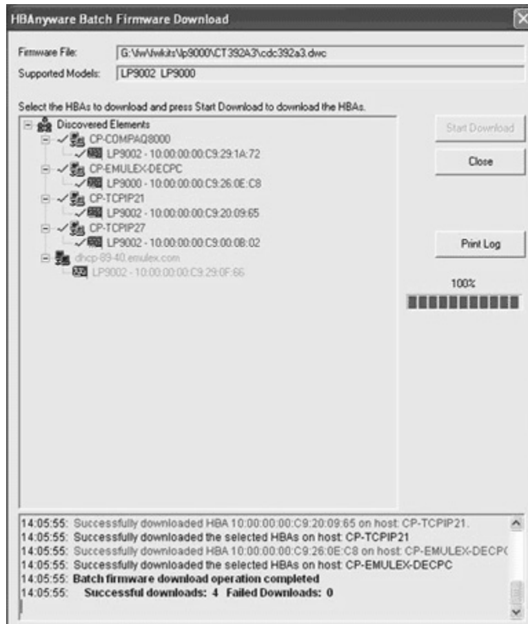
Figure 5: HBAAnyware Utility, Download Complete (Example)
