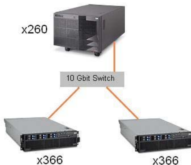
Figure 2: One server to two clients. A 10 Gigabit Ethernet switch is used to connect each system. Measurements were taken on the x260 server.
