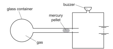
The mercury pellet moves and completes the circuit.
