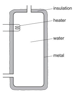
Water at the bottom of the tank stays cold for some time.
