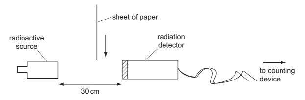
The experimenter moves the paper between the source and the detector. There is no difference in the count-rate.
