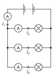
The currents measured with the ammeters are shown.
