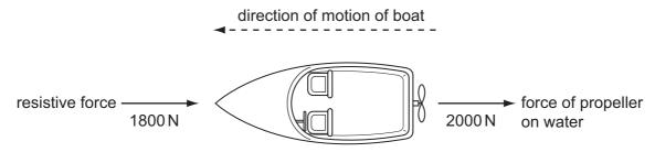
According to Newton's third law, what is the forward force on the propeller due to the water?
