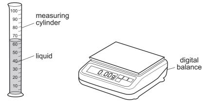
The student records the volume of the liquid from the scale on the measuring cylinder. He then puts the measuring cylinder containing the liquid on a balance and records the mass.
