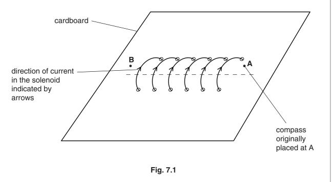
The plotting compass is used to follow magnetic field lines. On Fig. 7.1 draw in one magnetic field line which links **A** and **B**, both through the inside of the solenoid and round the outside of the solenoid. Mark the direction of each part of the field line with an arrow. [3] (b) Fig. 7.2 shows the result of a similar experiment with a current-carrying, straight wire.
