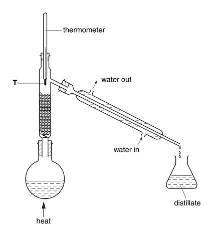
Which graph would be obtained if the total volume of distillate collected was plotted against the temperature at point **T**?
