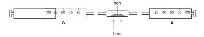
Syringe  $\bf A$  contained 80 cm<sup>3</sup> of air. The air was forced over heated iron into syringe  $\bf B$ . The air in  $\bf B$  was then forced back into syringe  $\bf A$ . The process was repeated several times until the volume of the gas forced back into  $\bf A$  was constant.
