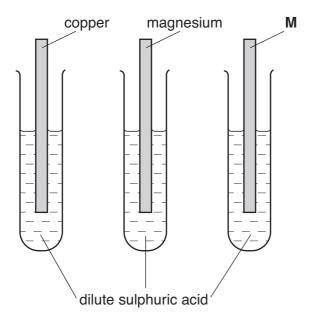
A gas was produced in **one** of the test tubes only.
