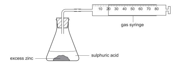
The same mass of zinc was used each time. The volume of acid used was different each time. Use the syringe diagrams to record the volume of hydrogen produced each time in the table.
