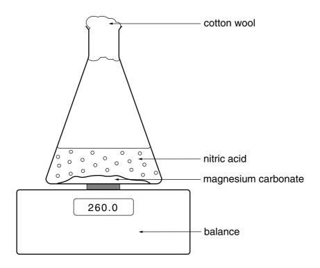
The flask was placed on a balance and the mass of the flask and contents recorded every minute. The results are shown in the table.
