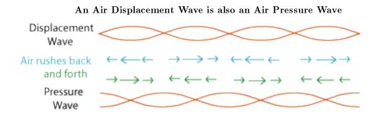
Figure 3.10: The nodes of the displacement wave, where the air is not rushing back-and-forth but is doing the most piling-up-and-spreading-out, are the antinodes of the pressure wave. The antinodes of the displacement wave, where the air is rushing back-and-forth the most, but is not piling up or spreading out at all, are the nodes of the pressure wave. Both waves must have exactly the same frequency, of course; they are actually just two aspects of the same sound wave.
