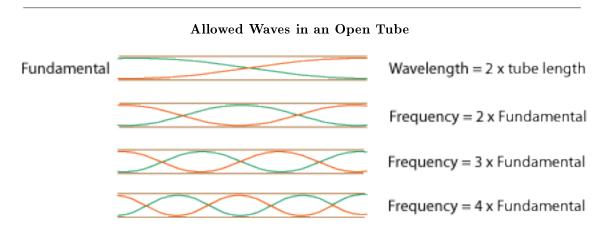
Figure 3.11: These are the first four harmonics allowed in an open tube. Any standing wave with a displacement antinode at both ends is allowed, but the lower harmonics are usually the easiest to play and the strongest harmonics in the timbre 46.
