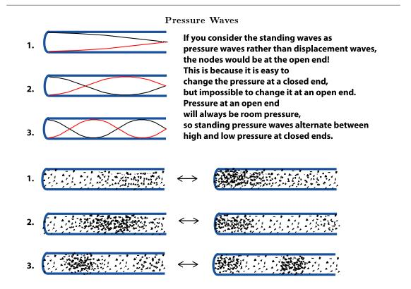
Figure 3.14: Here are those same three waves shown as pressure waves.
