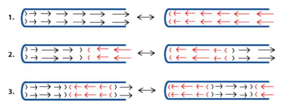
Figure 3.13: Here are the first three possible harmonics in a closed-open tube shown as longitudinal displacement waves.
