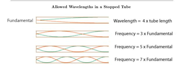
Figure 3.12: Again, these are the lowest (lowest pitch and lowest frequency) four harmonics allowed. Any wave with a displacement node at the closed end and antinode at the open end is allowed. Note that this means only the odd-numbered harmonics "fit".
