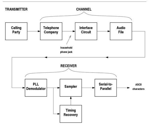
Figure 3.1: Caller ID decoder system to be constructed in this project
