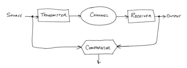
Figure 1.10: Generic communication system with comparator
