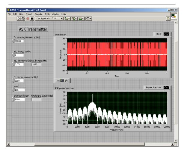
Figure 4.12: ASK transmitter VI front panel (click image to see fullsize version)
