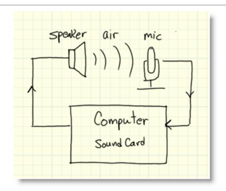
Figure 4.1: Speaker-air-microphone channel
