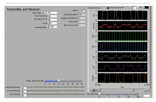
Figure 1.16: Suggested front-panel layout for TransmitterReceiver.vi
