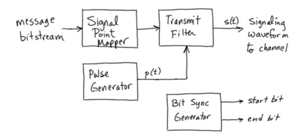
Figure 1.11: PAM transmitter block diagram
