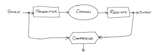
Figure 1.1: Generic communication system with comparator
