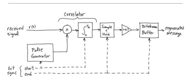
Figure 1.13: Block diagram of PAM receiver based on coherent detection
