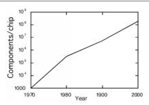
Figure 2.3: Number of transistors/chip
