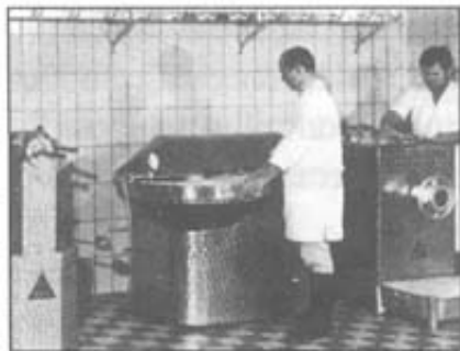
159. Processing in comminuting machines in medium-sized industries: grinder (right), cutter (middle) and filler (left)
